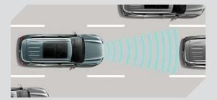
Automatically adjusts the speed to maintain a safe distance from vehicles ahead. The system uses sensors, such as radar or cameras, to detect the speed and distance of vehicles in front.
