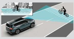
The Maxus D90 Max is equipped with Automatic Emergency Braking (AEB) feature to detect potential car crashes and automatically apply the brakes to avoid a collision or reduce the severity of impact. Whether in heavy traffic or open road.
