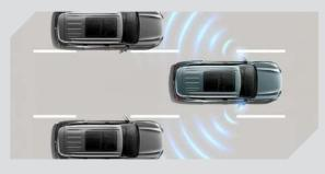
The Blind Spot System includes a range of technologies such as Blind Spot Detection, Rear Cross Traffic Alert, and Driver's Attention Warning. These features help to alert drivers of vehicles or obstacles in their blind spots, aiding in safe lane changes and preventing accidents.
