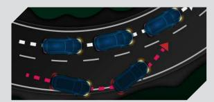
Helps to prevent accidents by detecting and reducing loss of traction. It automatically applies brakes to individual wheels and adjusts engine power to help the driver maintain control.
